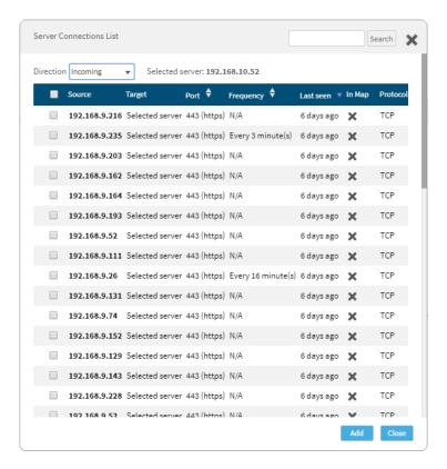
Switch between incoming and outgoing connections using the **Direction** drop-down menu.
