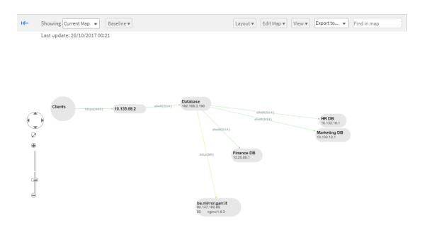
**Note:** The network topology data is collected every 4 minutes and stored for 24 hours. Data for servers and connections that have not been active for more than 24 hours is discarded and will not appear in the topology window.
