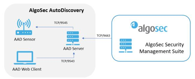
Traffic between AutoDiscovery components uses the following ports:
